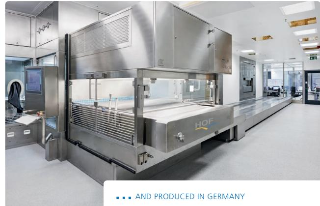
The loading and unloading systems are installed and tested in our own production area in combination with the freeze dryer or a specific equivalent dummy. All settings and functions can be tested extensively. This has the advantage that the installation and testing times are shorter at our customers site.
