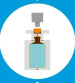
**SEALING** – Once the mandrel is removed, the head mould comes together to form the desired closure type.
