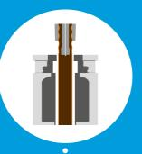
**EXTRUDING** – The polymer parison is extruded from granulate and positioned inside the open mould.
